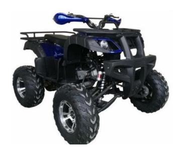
Pentora 250ccManual with Clutch- 4 Speed- Electric Start
